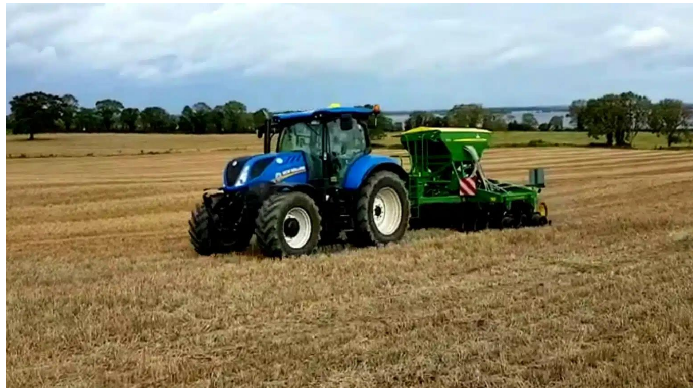
Image 5: Tractor with Direct Drill, planting crops on untilled soil
