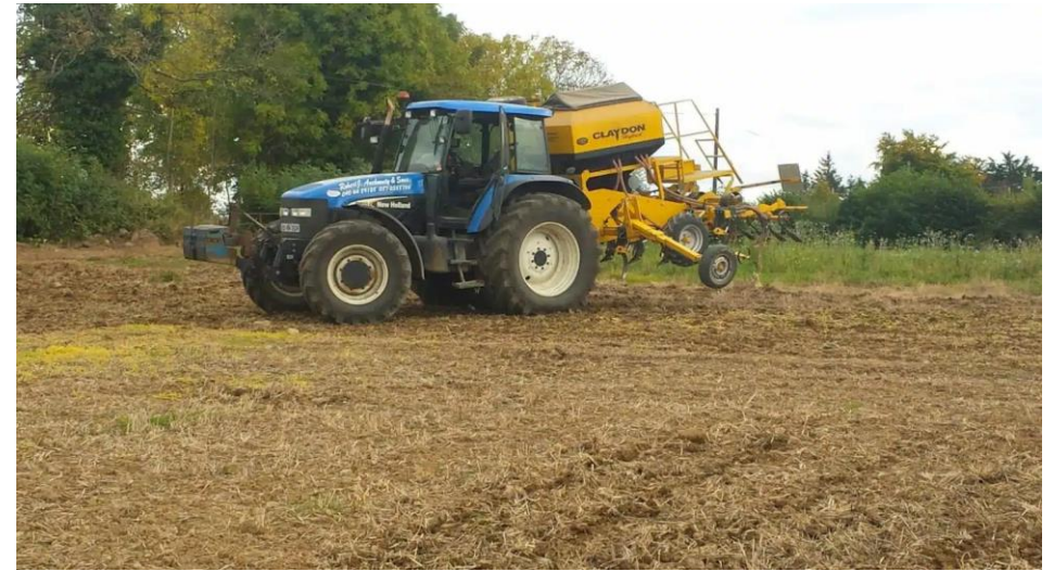
Image 6: Example of a Strip-Till Drill on unploughed soil
